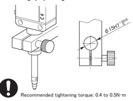
Mounting by squeezing stem using collar
