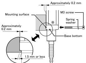
The mounting surface and base bottom of the sensor are made parallel and rectangular with the stem, respectively. Rectangular mounting can be accomplished easier by forming L-shaped lower end of the fixing jig.
