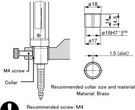
Recommended tightening torque:0.4 to 0.5N·m
