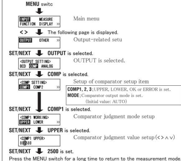
COMP1, 2, 3; UPPER, LOWER, OK or ERROR is set. MODE; Comparator output mode is set. (Initial value: AUTO)
