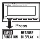
When the MENU switch is pressed in the measurement mode, the setup mode main menu is selected.
