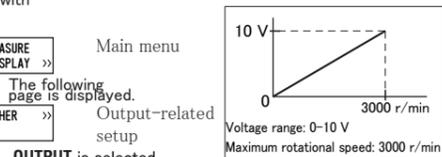
When the SET/NEXT switch is pressed in the state "0-ZERO", the cursor moves to "+0%". Adjust the analog zero value with the < > ▲ v switches. The setting range is 1-20% at a time; adjustable up to ±50% from the center.
