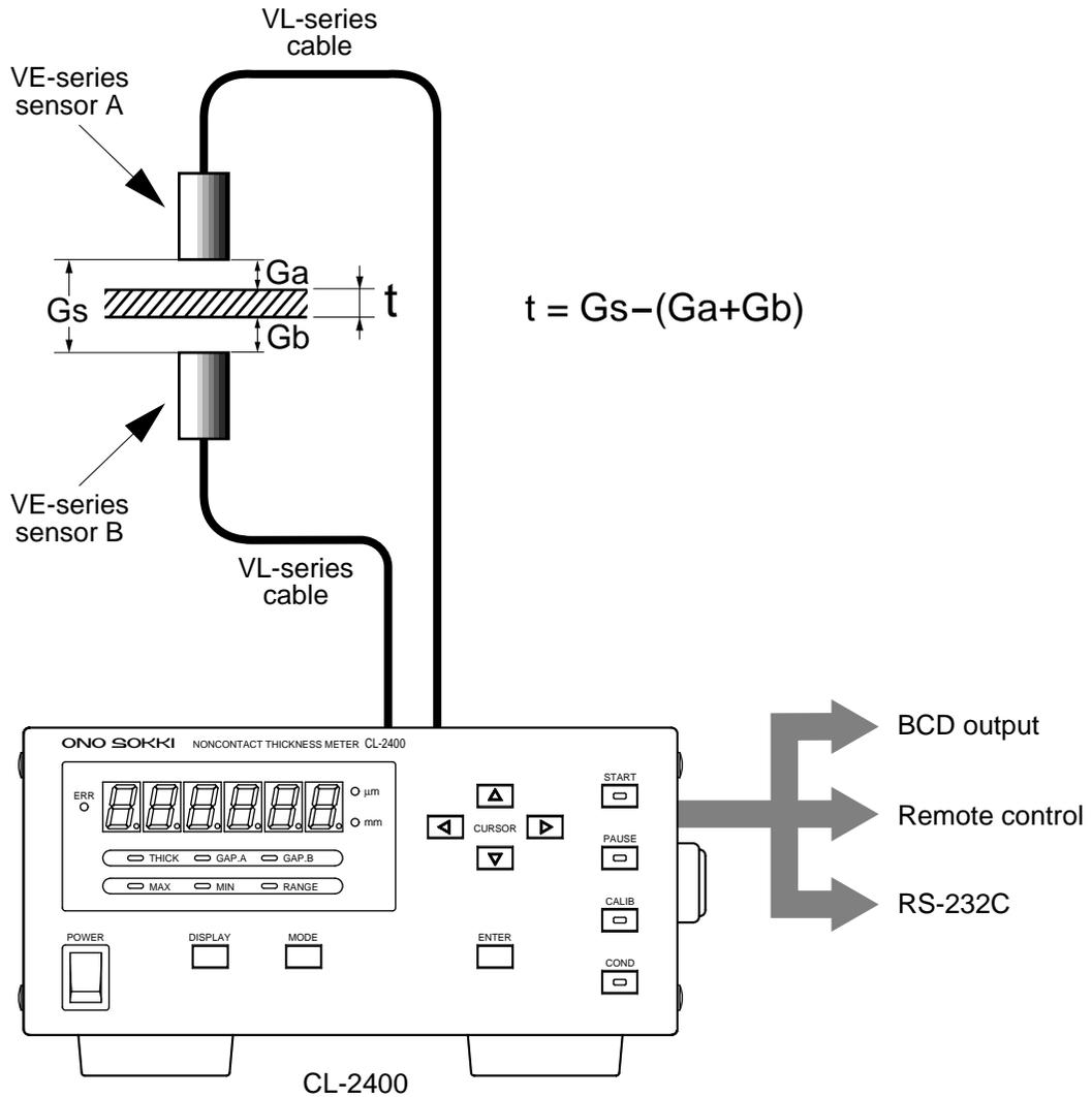
**Note:** This product has no overvoltage protection function for the sensors and sensor amplifiers due to its sensing mechanism. Trying to measure a charged object may destroy the sensor amplifier. Before starting the measurement, be sure to discharge the measurement objects with a discharging brush, discharging blower, etc.
