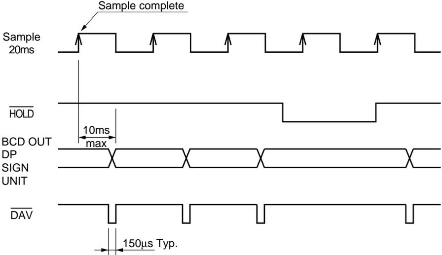
Note: Hold signal is recognized at the timing of sampling being completed. It takes 20ms max. to hold BCD OUT actually.
