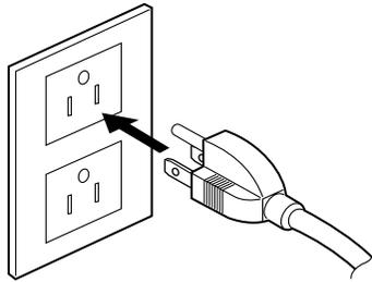
Insert the three-pronged plug into the three-position inlet.
