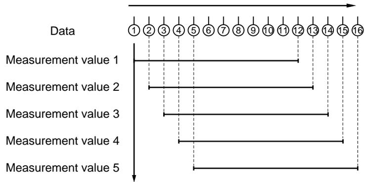
$$\begin{aligned} & \vdots \\ & \vdots \\ & \vdots \\ \text{Measurement value 1} &= \frac{\textcircled{1} + \textcircled{2} + \dots + \textcircled{12}}{12} \end{aligned}$$
