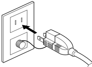
If no three-position inlets are available, use the attached adapter for grounding.
