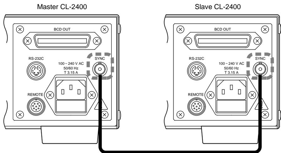
The master and slave CL-2400 units are connected at their SYNC connectors via a BNC cable.
