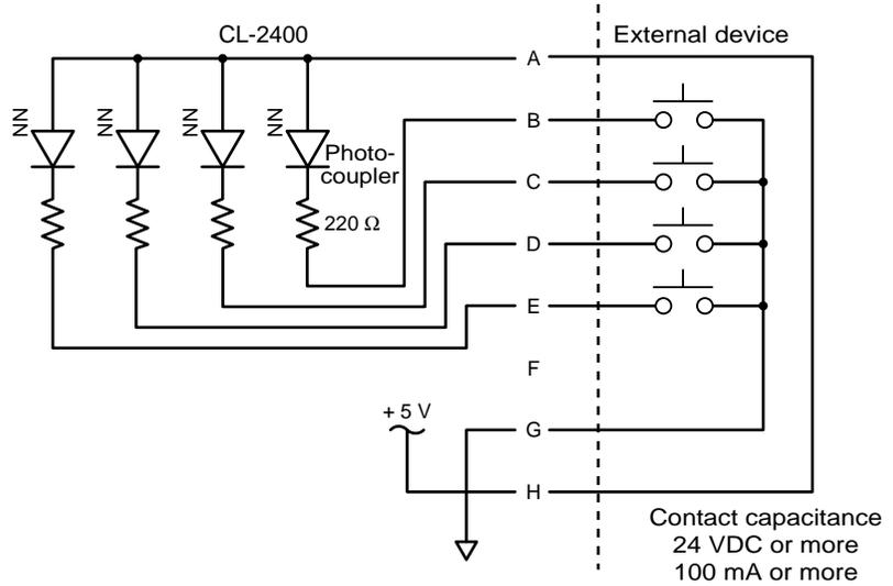
**Recommended interface 2 (when using internal power supply)**
