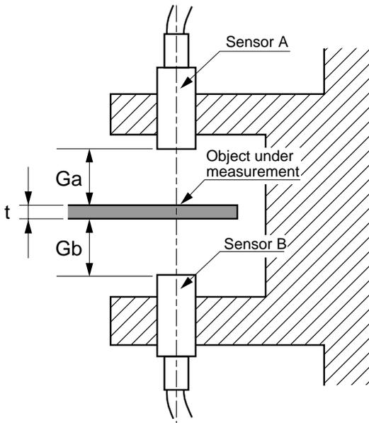
Mount the sensor securely so that the gaps ( $G_a$  and  $G_b$ ) between the sensors and measurement object are within the sensor gap ratings.
