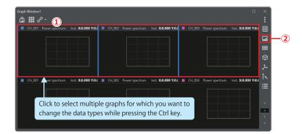
2. Change the data types of upper graphs (CH1 to CH3) to time axis waveform. When [Item settings] is displayed, select [Time axis waveform] (3) at [Data type].
