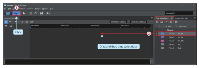
3. Check the waveform displayed at [Scope Window].
