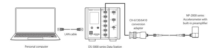
Case 3: Using Ono Sokki NP-3000 Series Accelerometer (with Built-In Preamplifier) or the Like and Ono Sokki PS-1300 Sensor Amplifier or the Like
