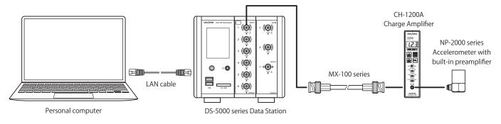
• For the case 3 and case 4, power is not supplied from the DS-5000 series Data Station to the sensor (CCLD disabled).
