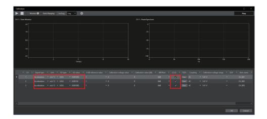
• With [CCLD] checked, +24 V/4 mA is supplied from the checked channel to the Accelerometer, and the signal is input correctly.
