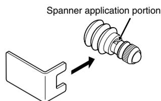
Rotate the probe by hand and then attach or detach it. When the probe is to be attached or detached using pliers, etc., apply a soft cloth to the probe to prevent the probe from being damaged.
